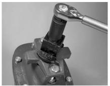
**2.** Loosen and remove the operator retaining nut from the end of the valve shaft.
