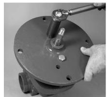
**6.** Reinstall and tighten the two mounting bolts.
