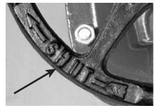
**1.** Install the handwheel onto the valve. Make sure "OPEN" and "SHUT" markings are facing up.
