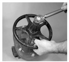
**2** Reinstall and tighten the operator retaining nut. To prevent the valve shaft from turning, restrain the handwheel.
