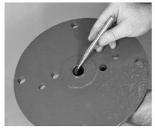
**4.** Inspect all seals on the valve and valve mounting flange. Replace damaged seals. Lubricate the seals using silicone or Victaulic lubricant.
