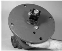
**7.** Reinstall the square operating nut onto the valve shaft. Reinstall and tighten the operator retaining nut onto the valve shaft to secure the square operating nut.
