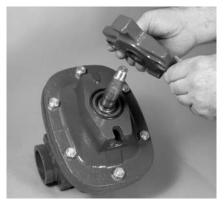
**3.** Remove the stem seal flange from the valve by lifting straight up off the end of the valve shaft.
