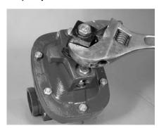
**1.** Fully open the valve by turning the square operating nut counterclockwise until you feel a sharp resistance.
