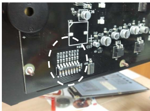
Figure 11 Microswitch situation at the back of the CPU circuit
