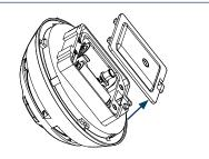
Remove the battery compartment cover on the base on the detector
