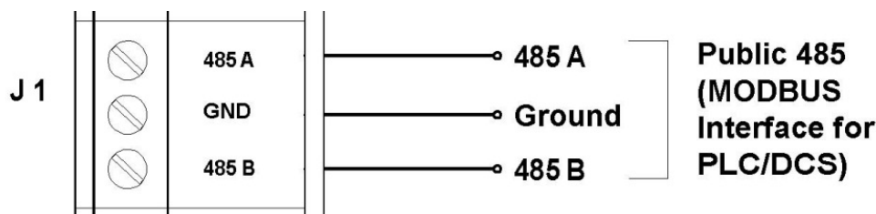
Figure 4-9 Wiring Diagram for the ModBus Interface
