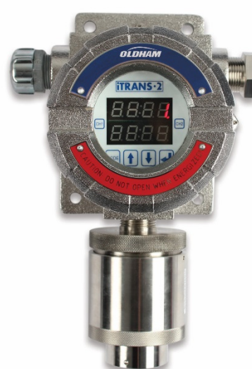
Figure 1-1 Typical iTRANS-2 Gas Monitor with Single Gas Sensor (Stainless Steel Option)
