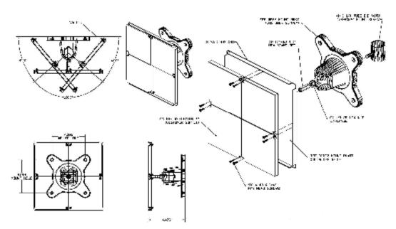
The 5000-007 Prism Alignment Adaptor comes pre-drilled to mount 4 Prisms (160 feet to 330 Feet) Designed to mount on the Alignment Adaptor 5000-005. Prisms and Alignment Adaptor 5000-005 are ordered separately
