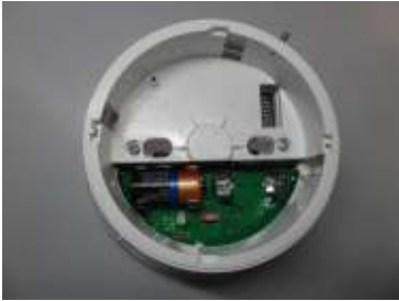
Picture 5 - secondary battery inserted
